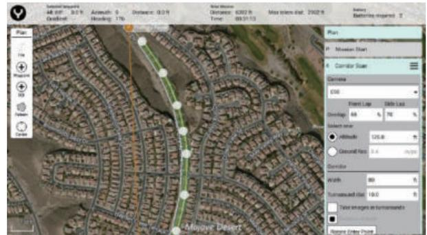
In this image, seven vertices have been inserted, allowing the Drone to follow the curvature of the roadway.
